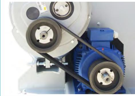
The wood-shredder works silent and poor in dust emission. The vibrations are reduced as much as possible by the use of a V-belt and the storage on special oscillating rubber elements. Electric motors of 18.5 up to 55 kW can be chosen as required and depending on the settings of tasks. The high performance helical gear unit works with high efficiency and we ensure 2000 working hours of warranty.
